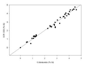
Figure 1. Scatterplot of % Si of fertilizer detected by ICP-OES versus molybdenum blue colorimetric analysis.
